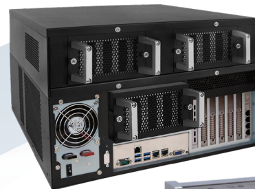
3x QuickTray®-v3 installed in the Mayflower®-Q12aW
