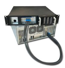
Example setup with a 4U system with host-card
