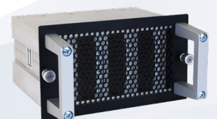
InoNet QuickTray® up to 14 GB/s* and 120 TB* with 4x NVMe-SSDs
